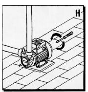
Never carry out any work on the pump without having first disconnected it from the mains supply.
